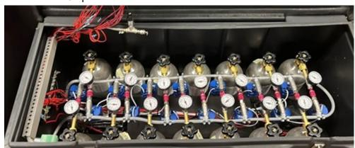
The Wireless Independent Noble Gas Samplers (WINGS) are inexpensive, autonomous, portable sampling systems that allow for multiple units to be placed in-field for improved temporal and spatial resolution.
