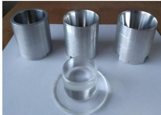
**Fig.6. measuring chambers and light guide.**
