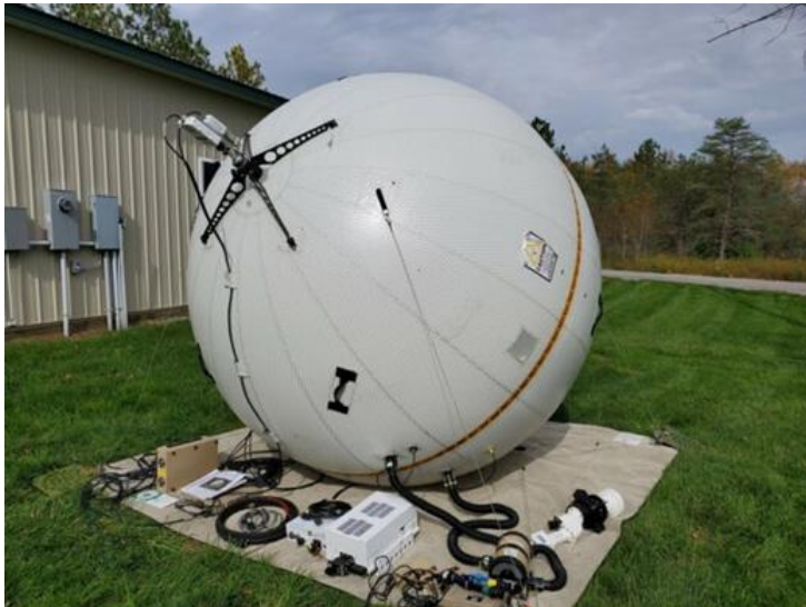
Inflatable VSAT antenna deployed in previous OSI field exercise
