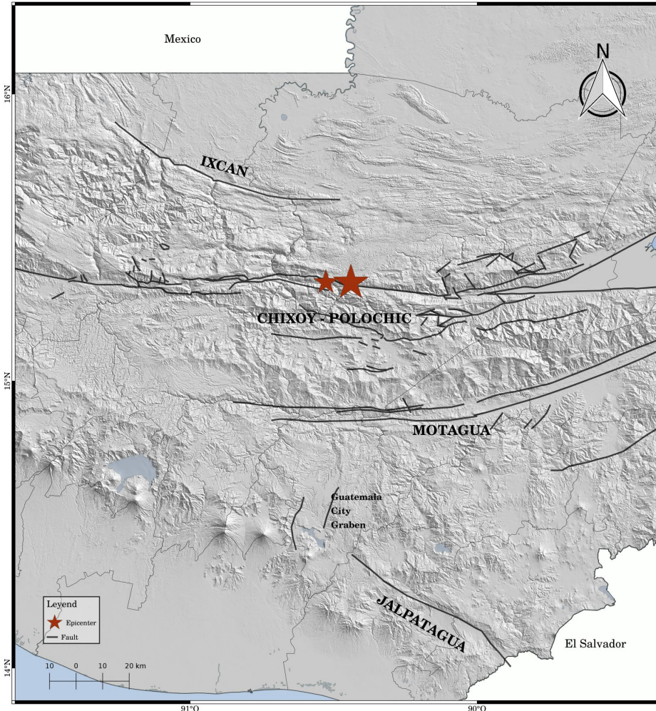
Figure 2. Detail of main seismic faults and epicenters of the January 2018 earthquakes in Guatemala.
