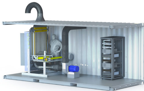
P3.2-746: Design drawing for an IMS type sampling system (manual or automated) utilizing electrostatic collections. A ruggedized prototype is planned to be tested by the developers in the next two years.
