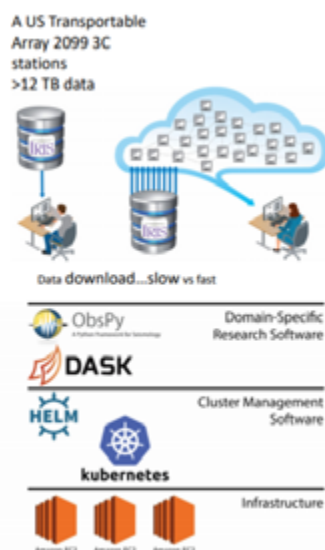
Figure 31. Custom designed research cluster in Amazon Web Services used for processing the large United States National Seismic Network dataset. G. A. MacLeod et al. [T4.3-P9]. More details here: J. MacCarthy, O. Marcillo, C. Trabant, Seismology in the Cloud: A New Streaming Workflow . Seismological Research Letters , DOI: https://doi.org/10.1785/0220190357
